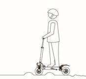
Do not ride at high speed on unconventional road, such as deceleration zone, lift threshold and uneven road. Keep at average speed (5~10km/h) on uneven road. You may get better adapted to roads mentioned above with knees slightly flexing.
