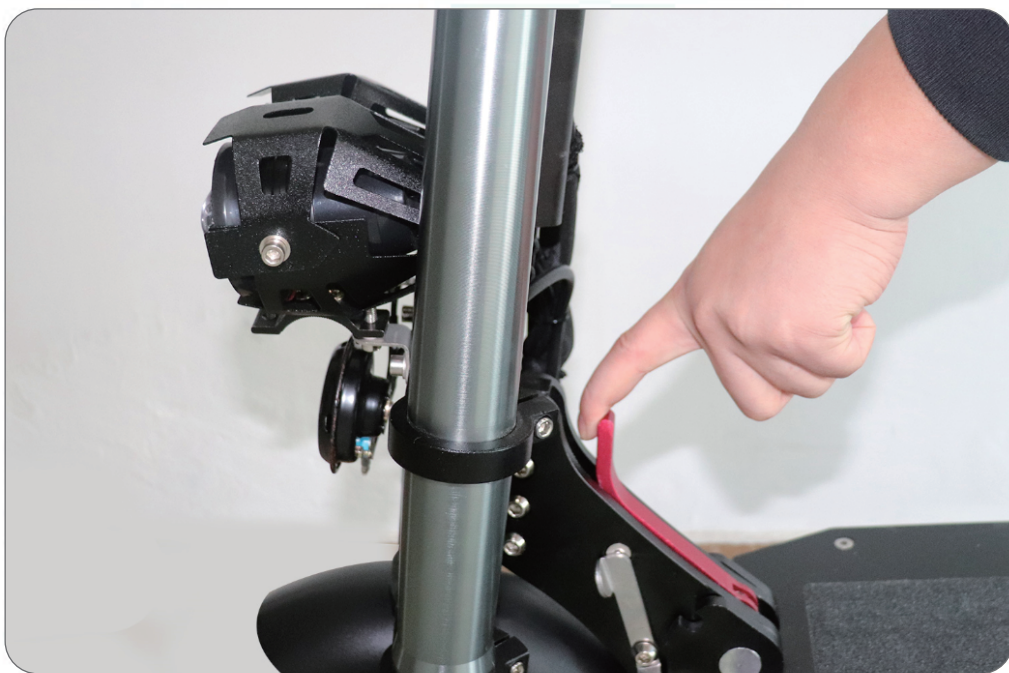
2. Press the lever lock switch to lock the lever
