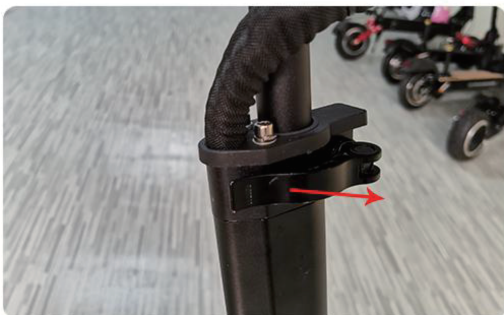
1. Open the lever to fix the buckle
