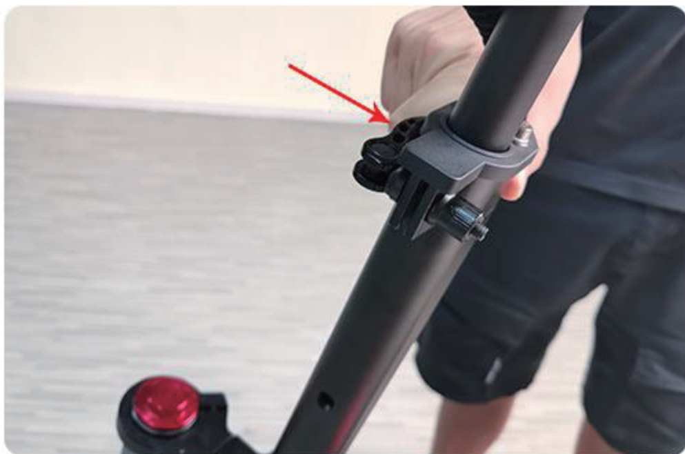
4. Press the lever lock switch to lock the lever
