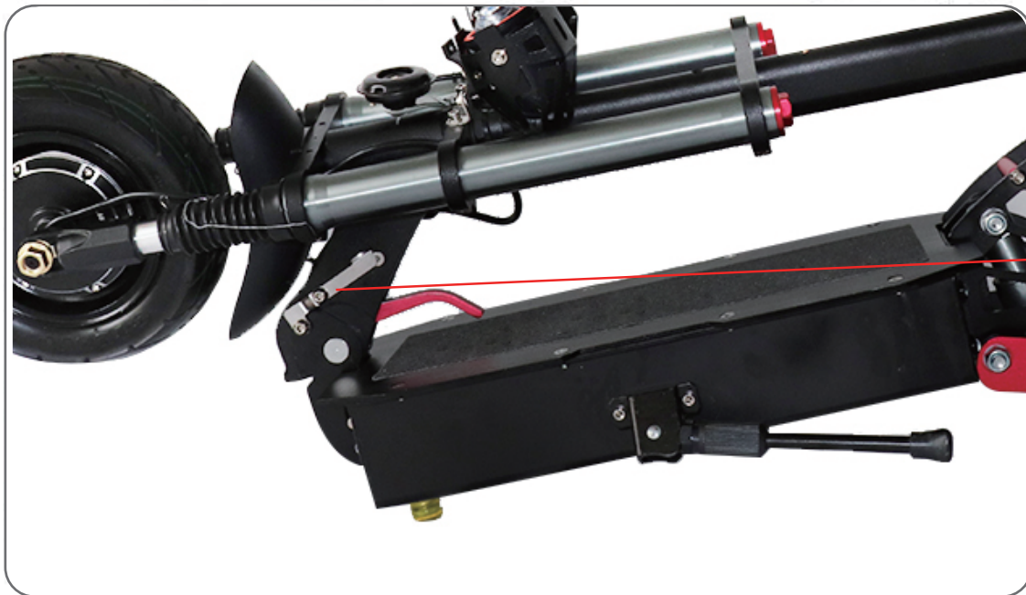
1. Press the folding switch to erect the rod
