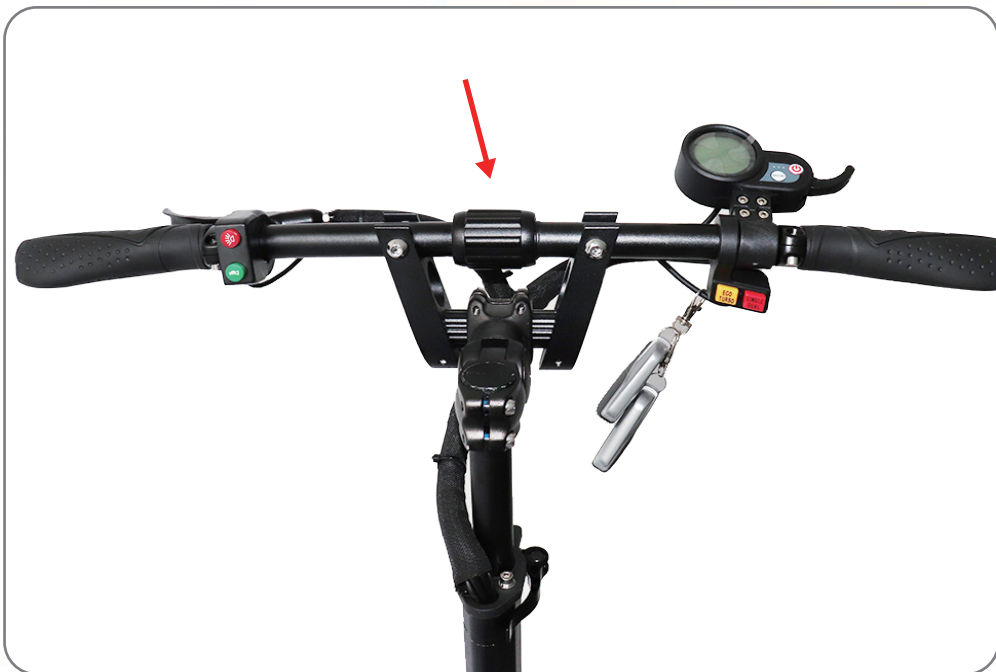
2 Rotate this position to fold the handlebar.
