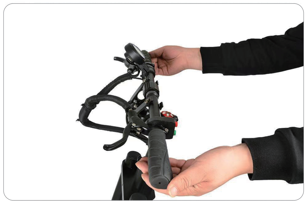
3. Lift the handle upward and unfold the handle
